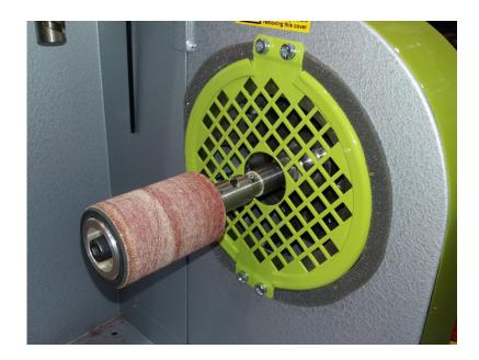
Tommy Bar to be inserted into hole on motor shaft to hold mechanism still. A short clockwise turn will loosed the tool from the machine.
