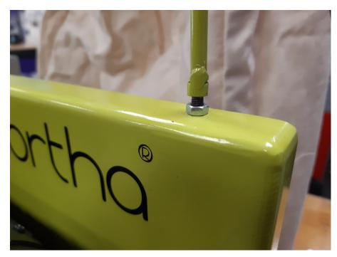
To remove the bag frame, loosen both the nuts holding the frame on.
